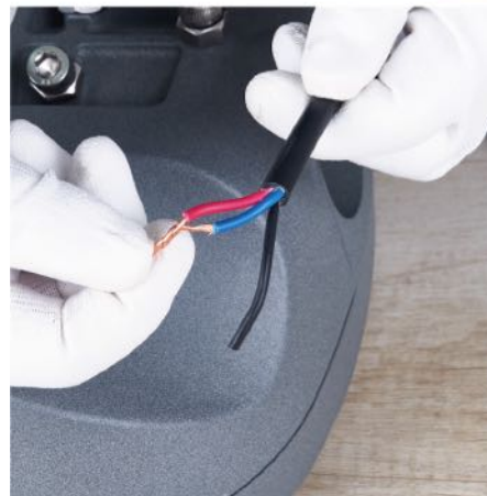
connect red line and blue line of the fixture together
