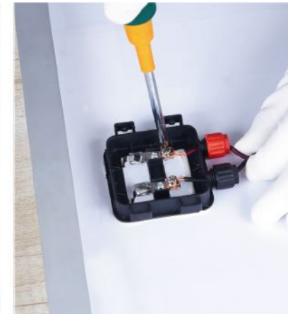
connect the cables with the solar panel
